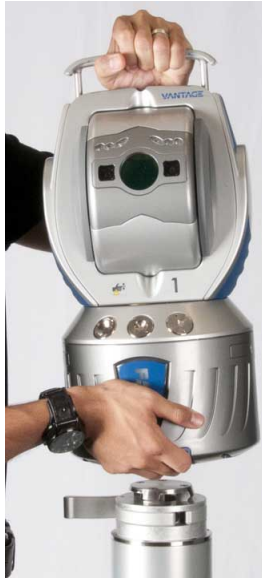
Figure 2-6 Mounting the Laser Tracker Measuring Head
