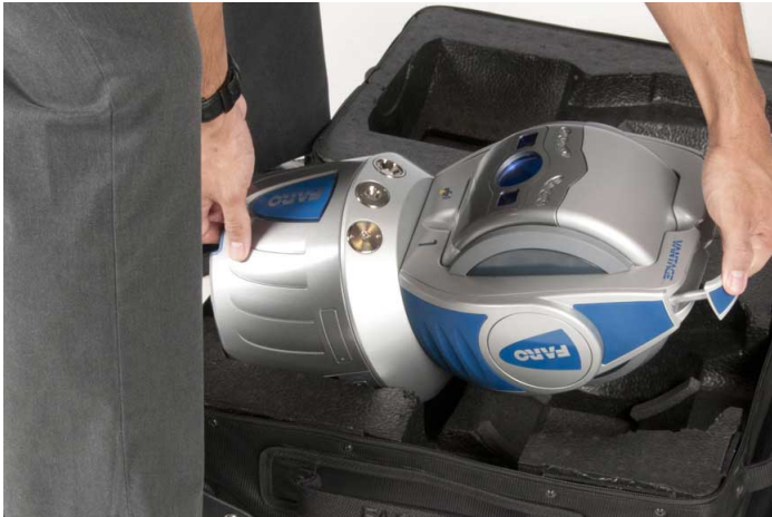
Figure 2-5 Lifting the Laser Tracker Measuring Head
