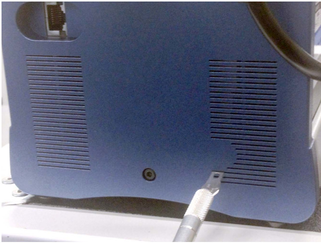
Figure 5-7 MCU Reset Switch Location
