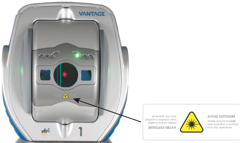
Figure 2-2 Laser Warning Labels on Aperture
