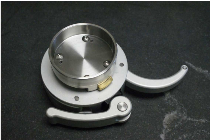
Figure 5-2 Tightening Side Lever
